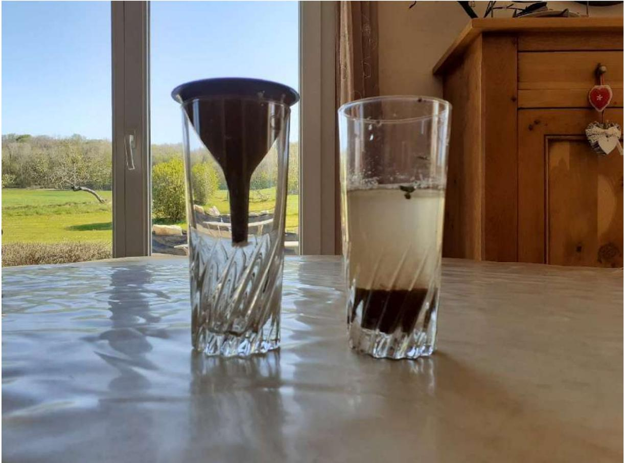
*Figure 2 PREPARATION DE LA FILTRATION (ENTONNOIR ET COTON)*
